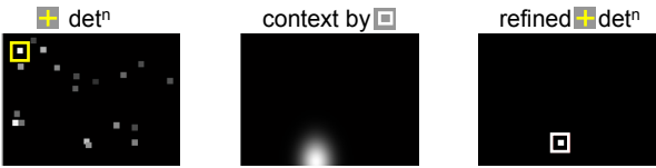
Figure 14. Left: candidate detections of keyboard, along with the max score (incorrect) detection. Middle: context prior provided by detected monitor. Right: detections of keyboard after applying context from monitor along with the max score (correct) detection. The centers of the candidate detections are shown.
