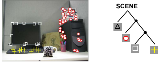
Figure 6. Results of the hSO learning algorithm. Left: The cloud of features clustered into groups. Each group corresponds to an object in the foreground. Right: The corresponding learnt hSO which captures meaningful relationships between the objects.
